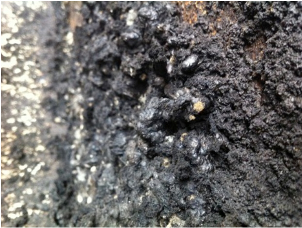
Fig 3. Hard, solid, carbonaceous debris such as this would likely be a poor candidate for sampling.
