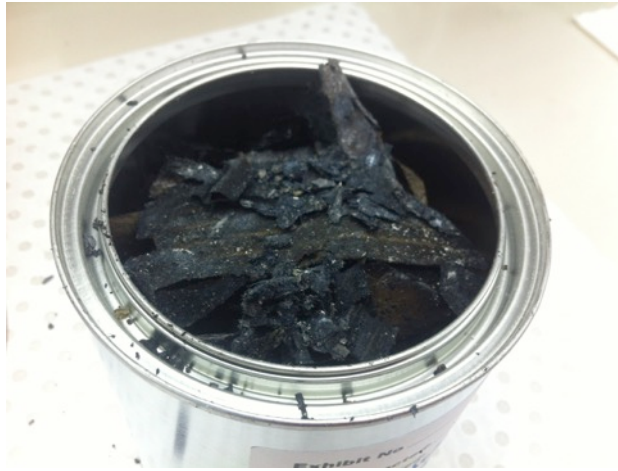
Do not overfill sample containers; this tin is too full.
