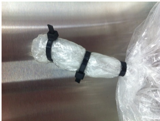
Well-sealed plastic bag: twisted shut, gooseneck tie, cable ties, and tape.
