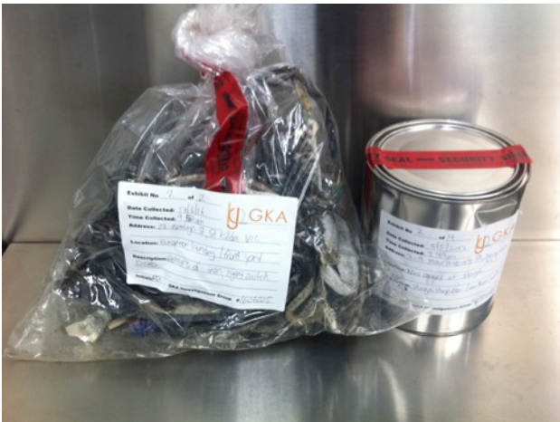
Appropriate fire debris packaging: metal tins and properly sealed fire debris bags.
