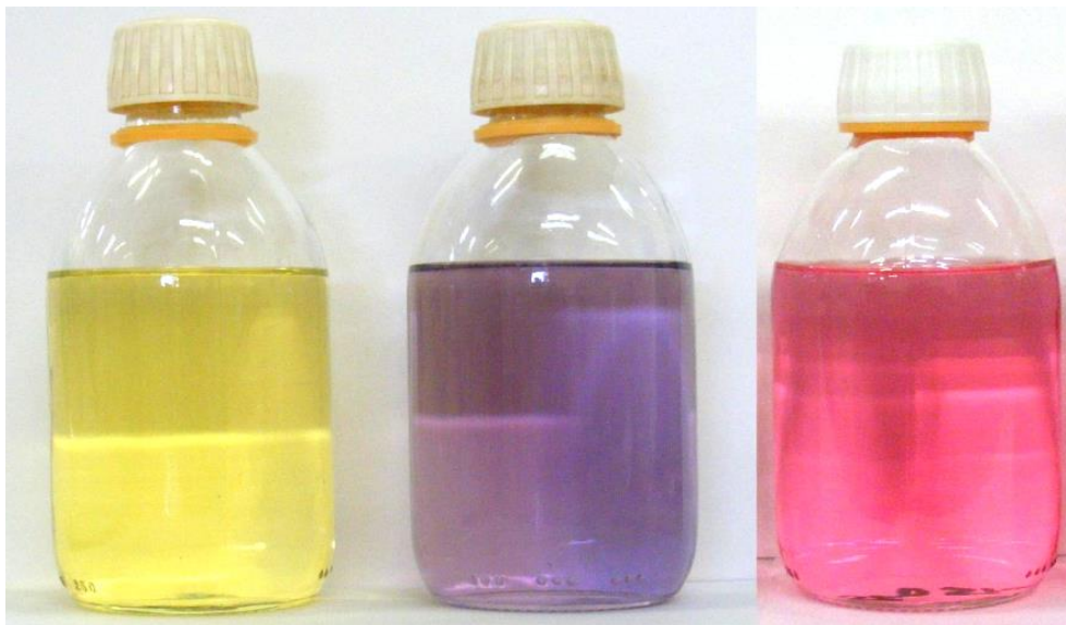
Figure 1: Colour of various unleaded petrol grades sold in Australia during 2012-2013. Left: premium unleaded petrol (yellow). Centre: 91 RON unleaded petrol up until October 2012 (purple). Right: 91 RON unleaded petrol after October 2012 (red). Source: AIP.
