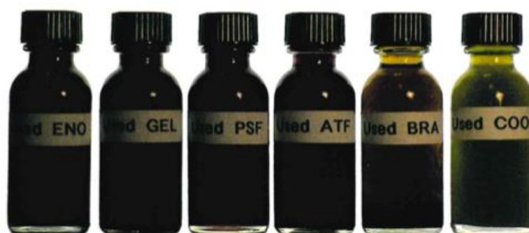
Figure 5: Depiction of the colours of various used vehicle fluids. From L-R: engine oil, gear lubricant, power steering fluid, automatic transmission fluid, brake fluid, coolant. Source: Stauffer et al.
